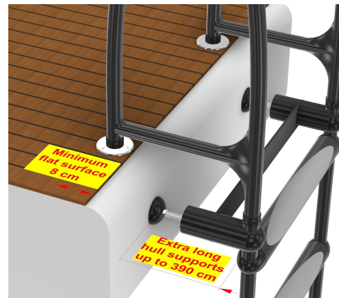
Mounting kit for a flat surface less than 17 cm long (minimum 8 cm), with the ladder farther than 15 cm from the hull: Standard Sockets plus "Extra long, stabilized hull support", to be added as an option according to the distance between ladder and hull, and respecting the width of your ladder
